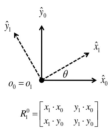
1. the rotation matrix  $R_j^i$  can be interpreted as the orientation of frame  $\{j\}$  expressed in frame  $\{i\}$
